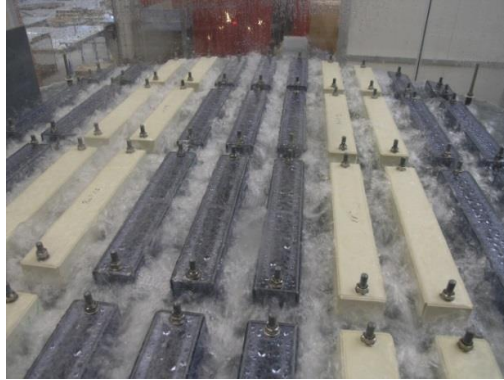
Tray column equipped with tunnel trays in operation P114_RVT_TestFacilities_pic2
