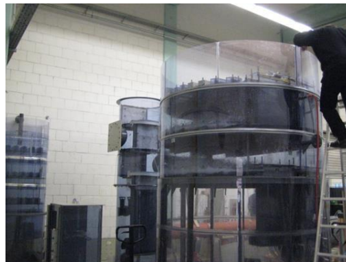
Tray column Ø 1,500 mm P114_RVT_TestFacilities_pic3
