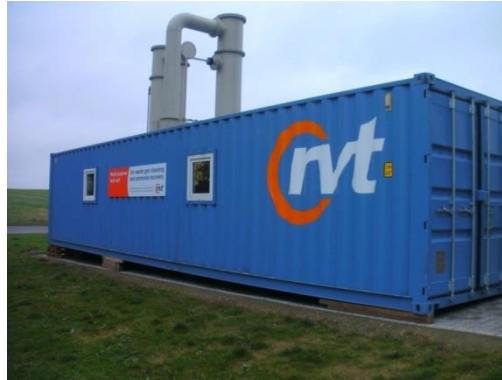
Mobile multi-purpose plant for ammonia stripping and waste gas scrubbing ready for start-up with mounted columns for stripping and absorption P114_RVT_TestFacilities_pic5
