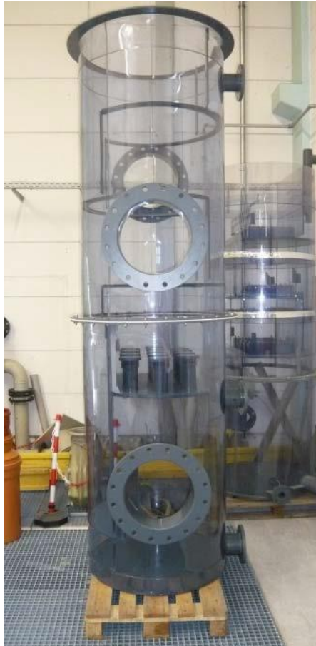
Tray column Ø 900 mm P114_RVT_TestFacilities_pic1
